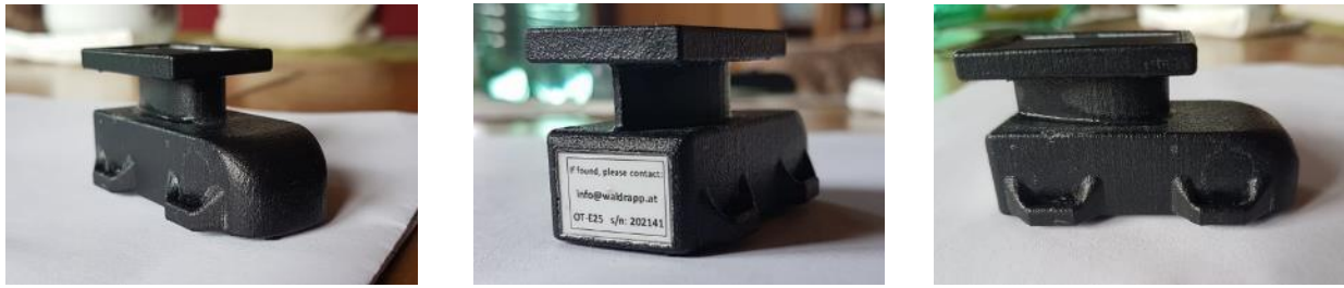
Figure 1 a-c: Pictures of the OrniTrack-E25 transmitter with adaptation of the bridge and four lateral attachment points, used in the “LIFE Northern Bald Ibis”-project.
